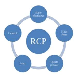
RPCs have an ultra-dense microstructure, giving advantageous waterproofing and durability characteristics. These materials can therefore be used for industrial and nuclear waste storage facilities. RPC has ultra-high durability characteristics resulting from its extremely low porosity, low permeability, limited shrinkage and increased corrosion resistance. In comparison to HPC, there is no penetration of liquid and/or gas through RPC.
