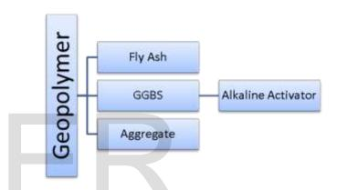
Compressive strength of geopolymer concrete have been found up to 70 MPa (N/mm2). The concrete gains its compressive strength rapidly and faster than ordinary Portland cement concrete. The concrete strength after 24 hours have been found to be more than 25 MPa. Compressive strength after 28 days has been found to be 60 to 70 MPa.
